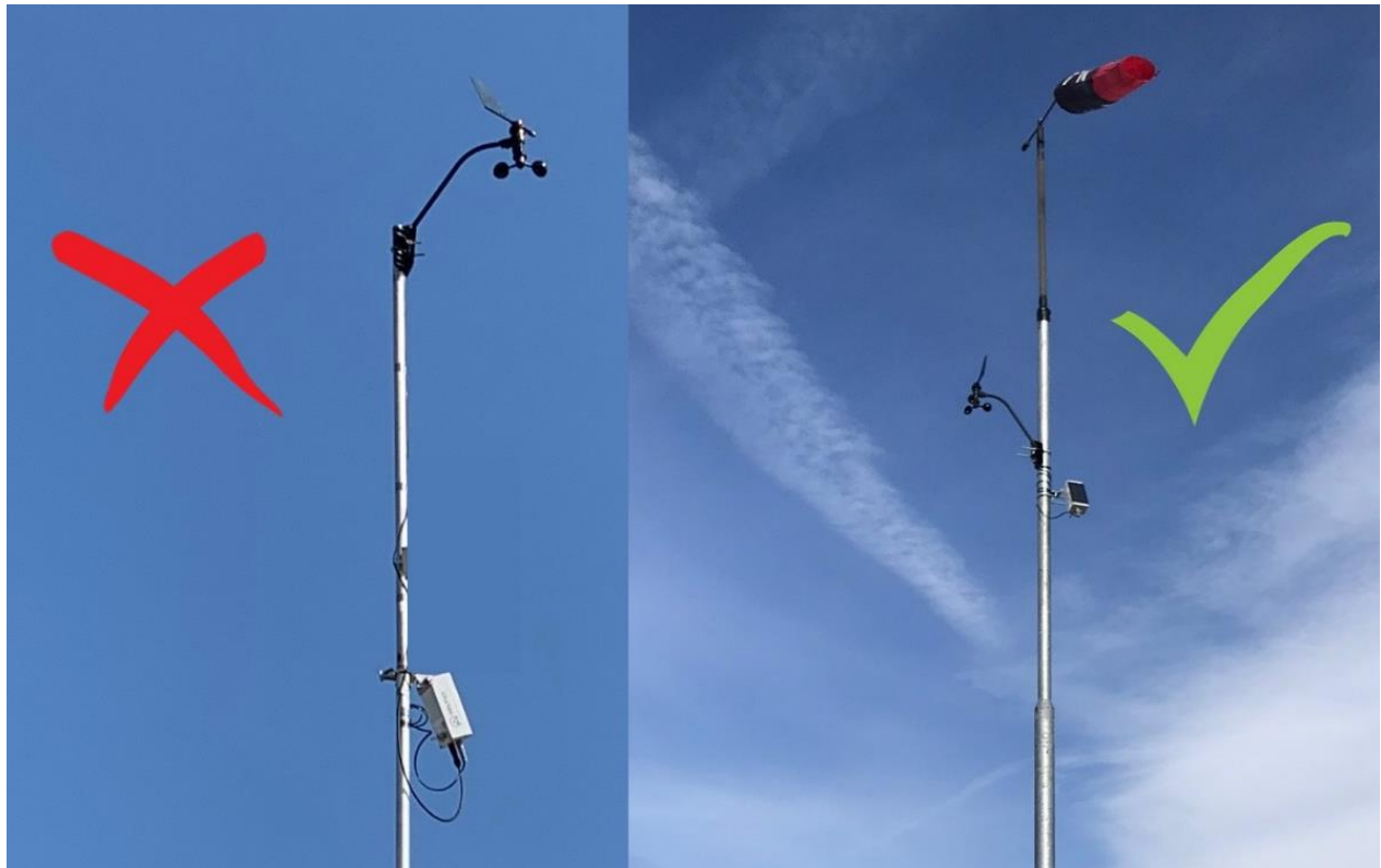
Mounting of the wind sensor: proper (right), wrong (left, as wind sensor is at the highest point)
